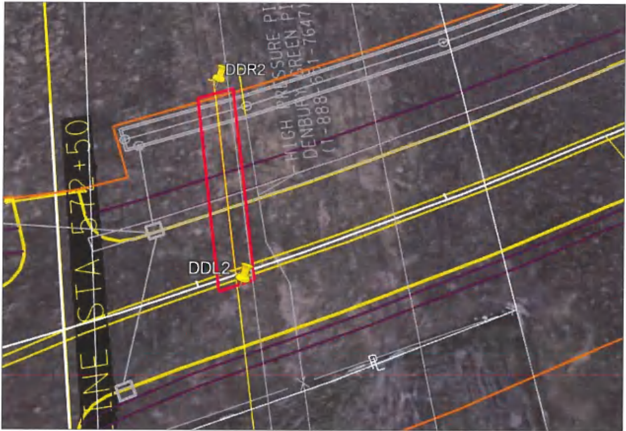
Figure 2. Drainage ditch conflict approximately 123 ft. in conflict.
