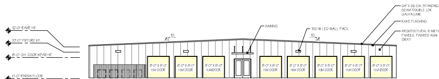
4 WEST ELEVATION - BLDG. C SCALE: 3/32"=1'-0"
