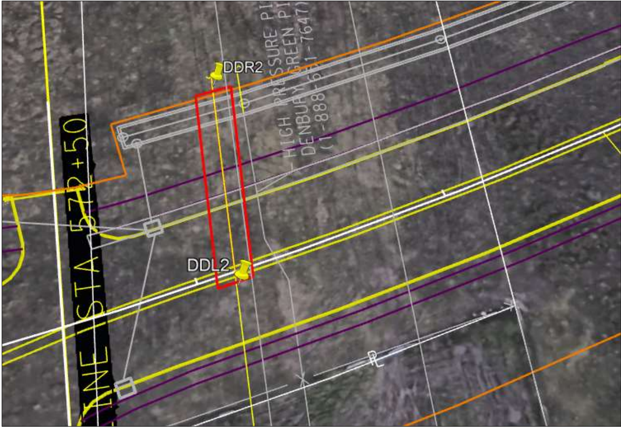
Figure 3: Drainage ditch conflict approximately 123 ft. in conflict.
