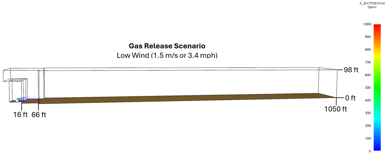
Figure 21: The model for a non-fire scenario with no ventilation and low wind speeds. X_BATTERYGAS is the concentration of battery vent gas in ppm. The distances shown are measured from the front of the enclosure.
