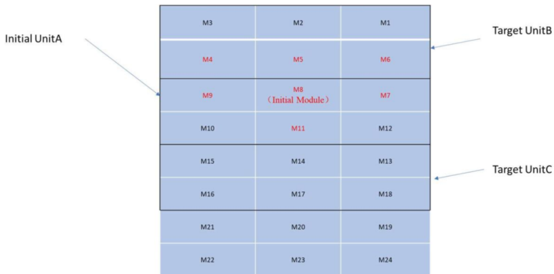
Figure 16: The initiating unit with the initiating module and target modules labeled. This image was taken from the UL 9540A unit-level test report [8].
