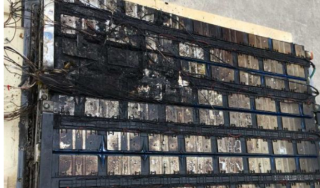
Figure 15: The internal contents of the module after the UL 9540A test. This image was taken from the UL 9540A module-level test report [7].
