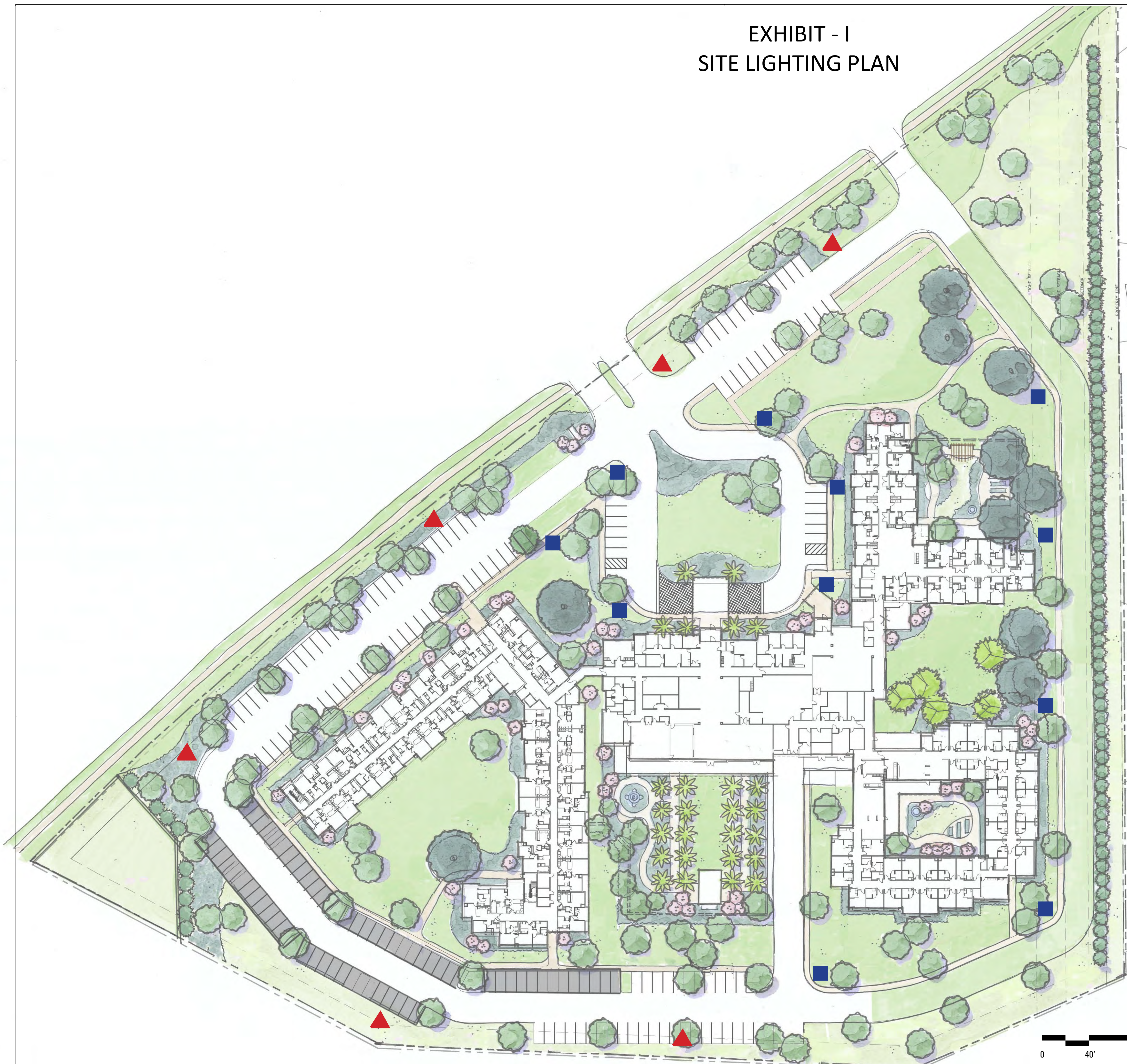
PARKING LOT FIXTURES LITHONIA D SERIES LED 25' POLE HEIGHT 250' APPROX. SPACING
