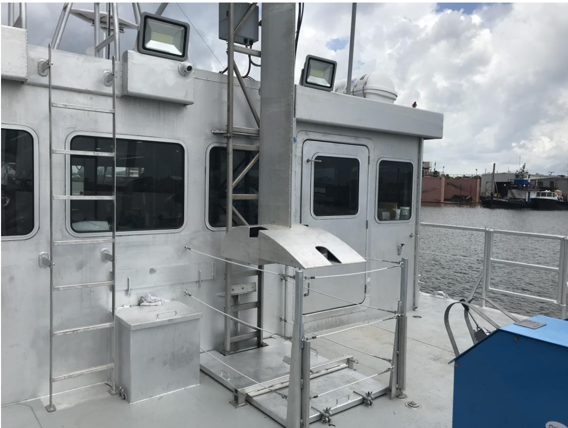
POD in the up position with the Moon pool hatch in place and secured.
