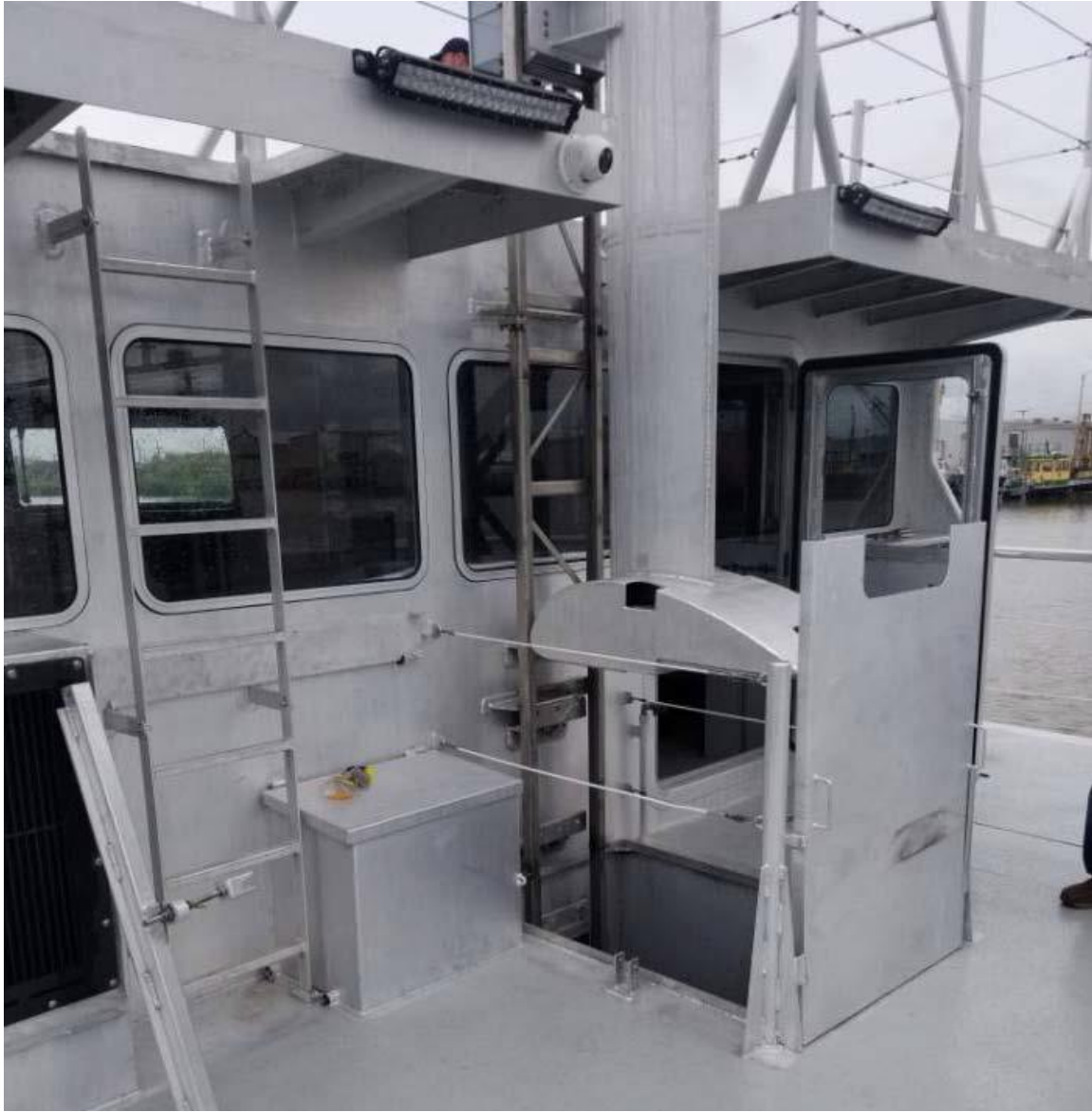
POD in the up position with the Moon pool hatch in the stowed position.
