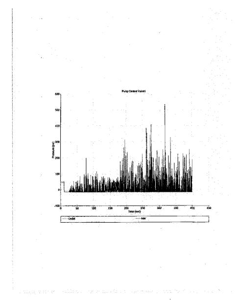
Graph A – Pressure Surges at the Pump Control Valves without Surge Controls (i.e., no AIV's)
