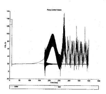
Graph D - HGLE Surges at Pump Control Valves with Recommended Surge Controls Installed
