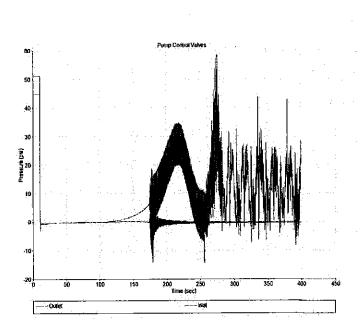
Graph C – Pressure Surges at Pump Control Valves with Recommended Surge Controls Installed
