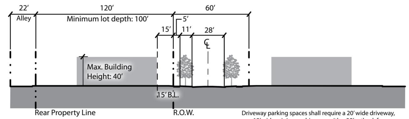
Driveway parking spaces shall require a 20' wide driveway, or a 12' wide minimum driveway with a 35' setback from the edge of right-of-way.
