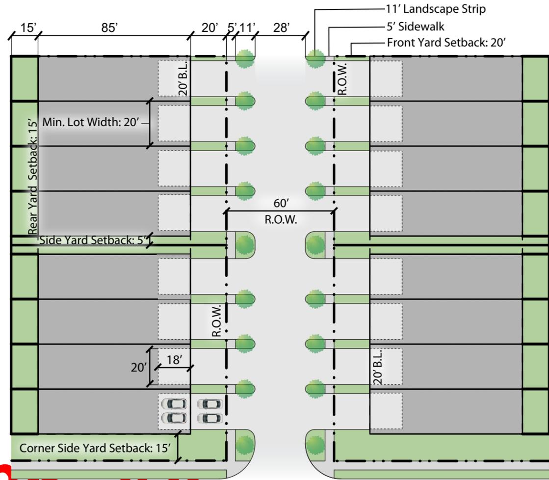
Note: Driveway parking spaces shall require a 20' wide driveway of a 12' wide minimum driveway with a 35' setback from the edge of right-of-way.
