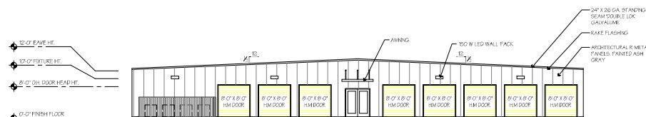
4 WEST ELEVATION - BLDG. C SCALE: 3/32"=1'-0"
