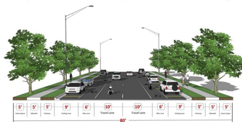
Collector – 2 Lane, 80' ROW, 10' Travel Lanes, 6' Bike Lanes & On-Street Parking
